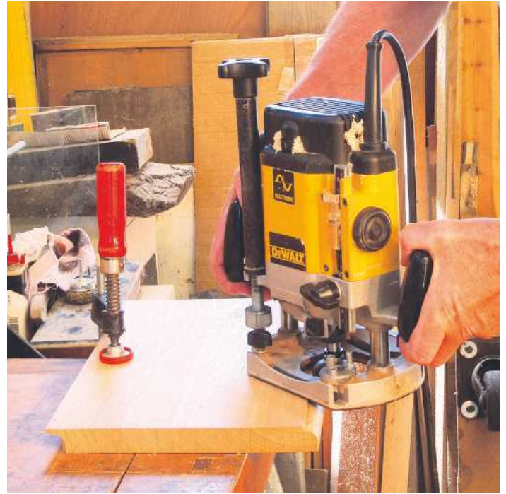
▲ Pic.8 A larger leaf has to be cramped to the bench
